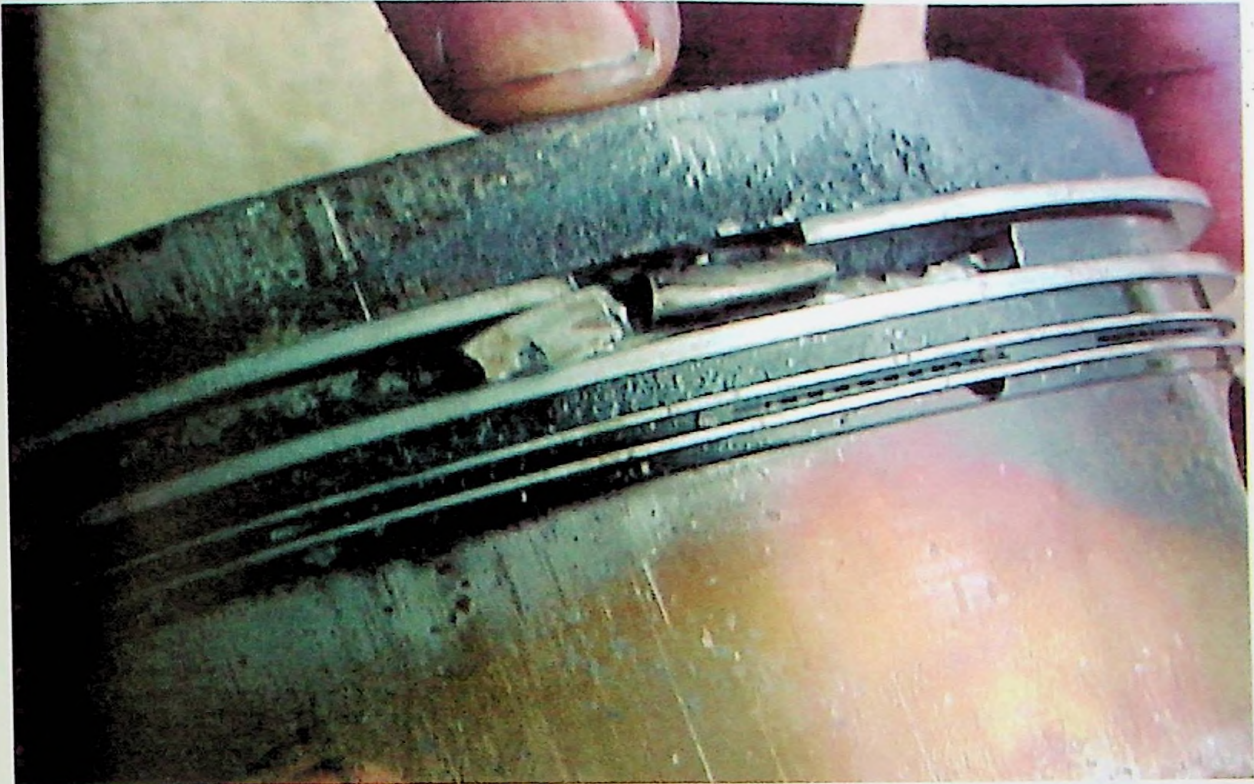
The number 3 piston showing the damaged top compression ring-land.
