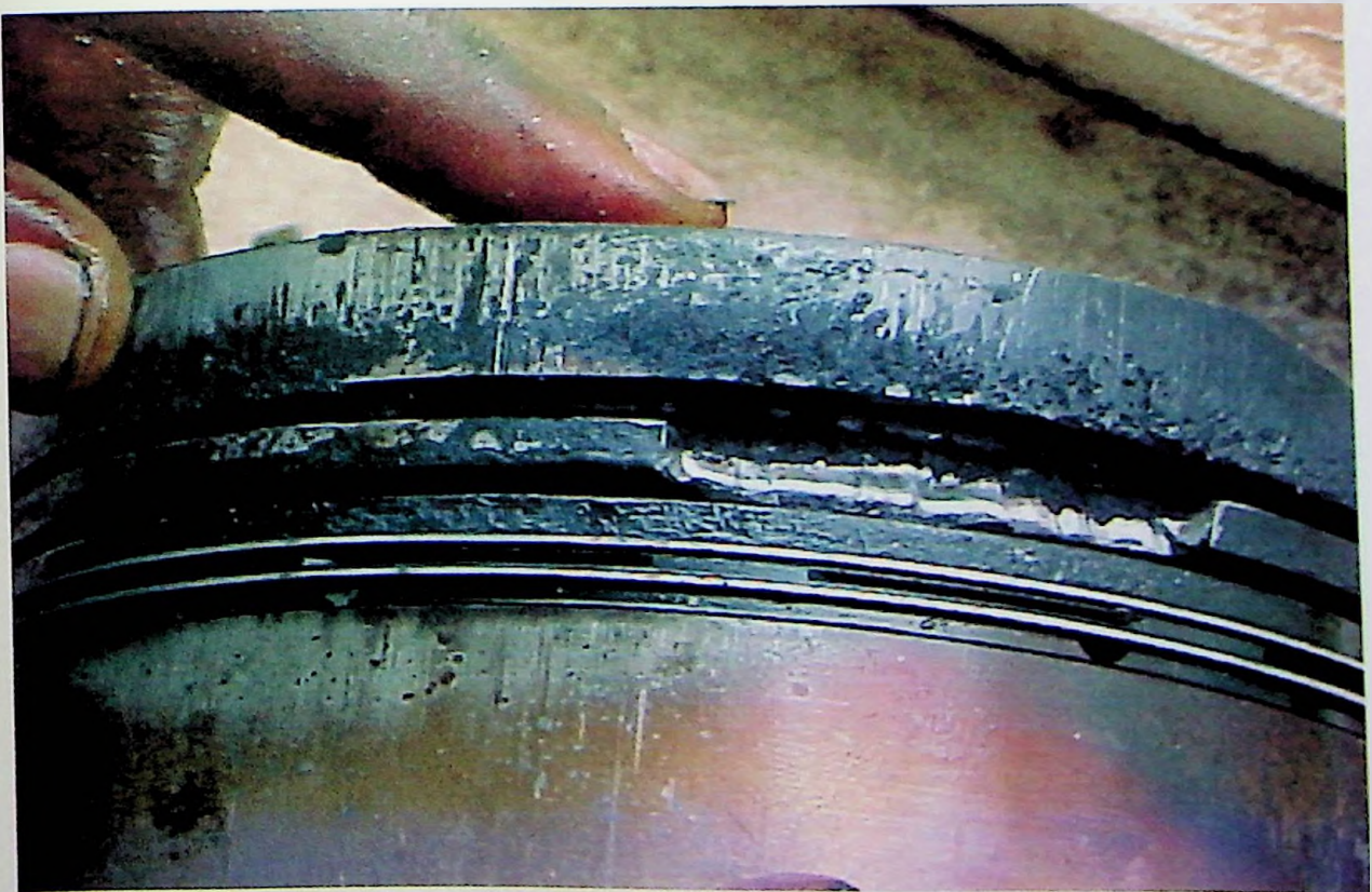
The close-up picture of the top compression ring-land and the carbon deposit.
