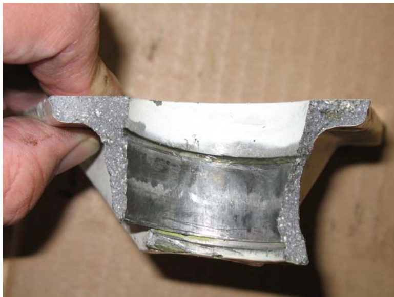
Front fitting, fracture.
