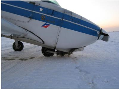
Figure 1: Bent nose wheel leg.
