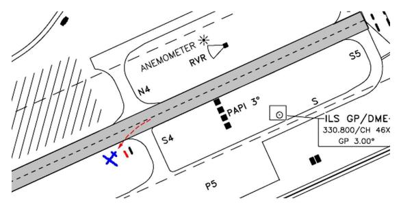
Red arrow: estimated trajectory of the plane Black line: signalisation board S4 - initial position Red line: signalisation board S4 - final position after impact (approx. 4m from initial position)
