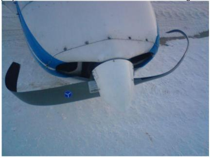
Figure 4: Bent propeller due to impact with ground.
