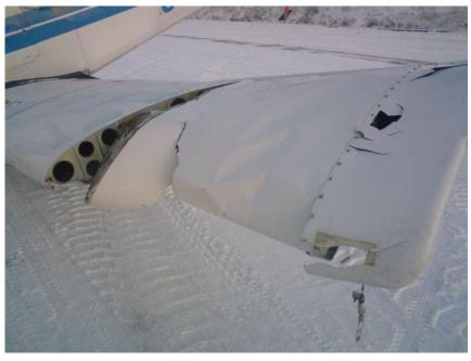
Figure 3: Damaged left wing spar.
