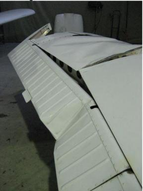
Figure 2: Damaged flaps and ailerons on left wing.
