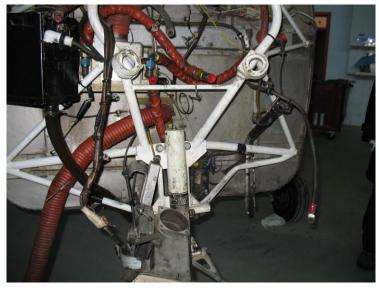
Figure 5: Dented engine support assembly.
